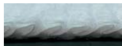
Easy to notice: The cross section illustrates that the waved structure offers a much larger filtration surface in the same dimensions as usual flat media.
