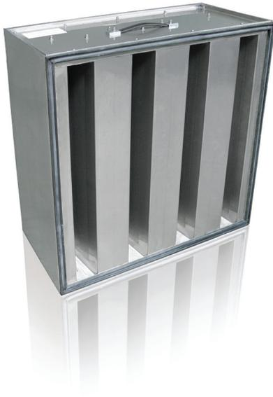
This exchangeable carbon cell is highly efficient within incoming air as well as exhaust air systems that hold high degrees of gases and odours. It is especially equipped to extract radioactive gases such as iodine, its compounds as well as war gases. It is originally designed to serve within nuclear facilities. The compact retainer cell is made from stainless steel (1.4301). Precisely welded perforated sheets plates fix the 50 mm thick layer of activated carbon into place.
