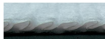
Easy to notice: The cross section illustrates that the waved structure offers a much larger filtration surface in the same dimensions as usual flat media.
