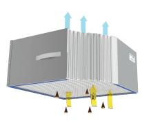
Absorbed oils and fluids are constantly released from the filter by gravity.
