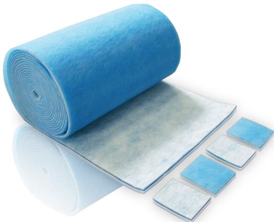
These HS-synthetic filter pads consist of synthetic-organic polypropylene fibers, which are non-breakable. They may be installed into HVACs and ventilation systems as well as ceiling fans and cabinets for machines. The design consists of randomly arranged synthetic fibers. Its density increases progressively towards the clean air side of the media. This specific structure of non-coated filtration mats ensures a high retention capacity towards dust with low pressure differences.
